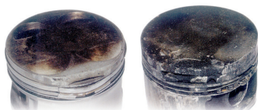
Pistons damaged by detonation.
